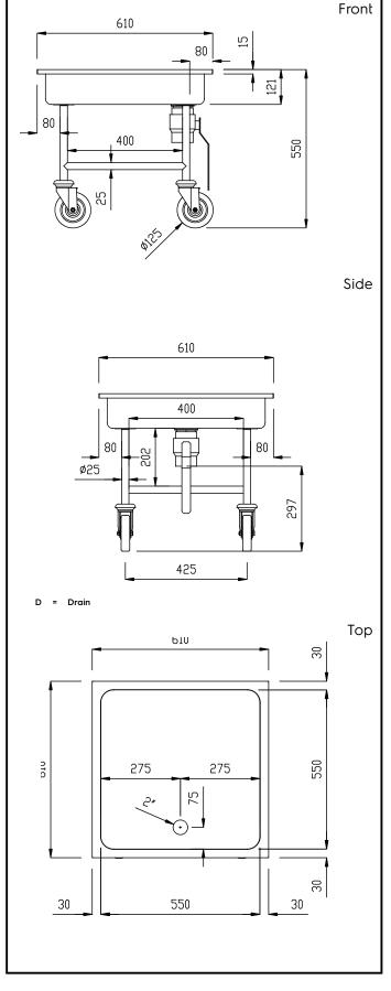
Service Trolleys Soaking Sink Trolley for Cutlery - 610 mm
